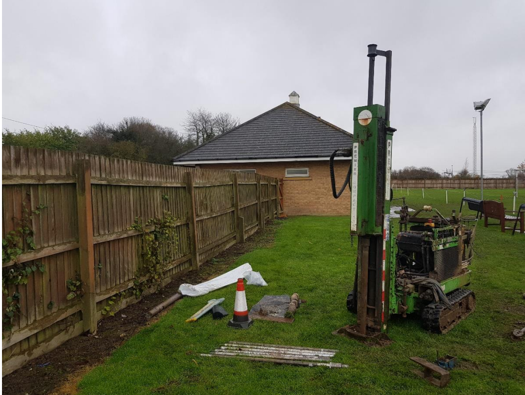
Photo 7: Window sampling rig drilling in BH2
