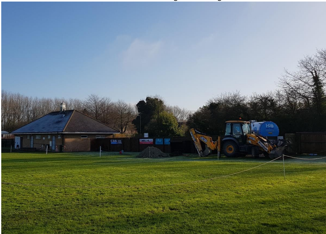
Photo 4: JCB 3CX and Water Bowser conducting BRE soakage test onsite
